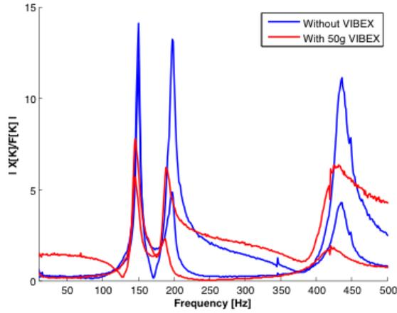
Figure 11: FFT of all Sensors (Impact location -4, at the rear end of the holder)
