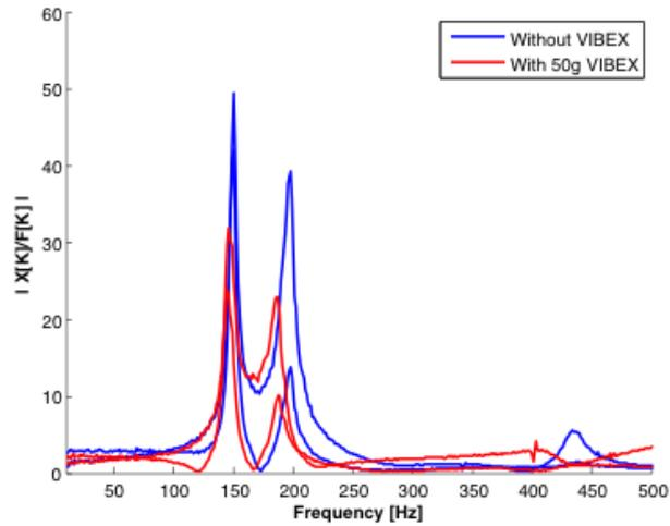
Figure 10: FFT of all Sensors (Impact location –3, at the rear end of the blade)
