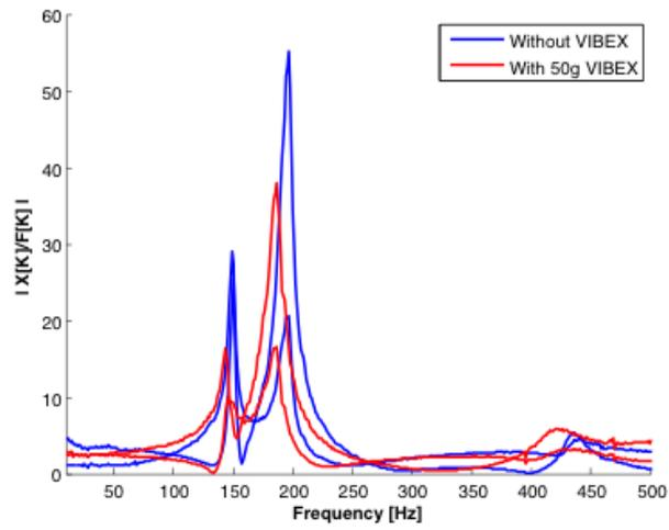
Figure 8: FFT of all Sensors (Impact location – 1, at the front end of the blade)
