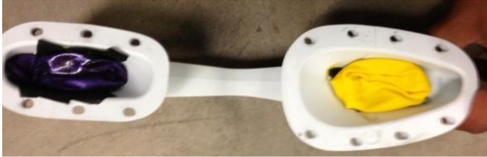
Figure 2: Easton Mako CXN blade holder with VIBEX Sport in the bladders (purple and yellow color balloons in figure have 15g of VIBEX Sport)
