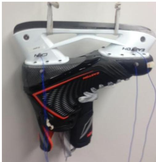
Figure 1: Easton Mako CXN skates suspended with accelerometers
