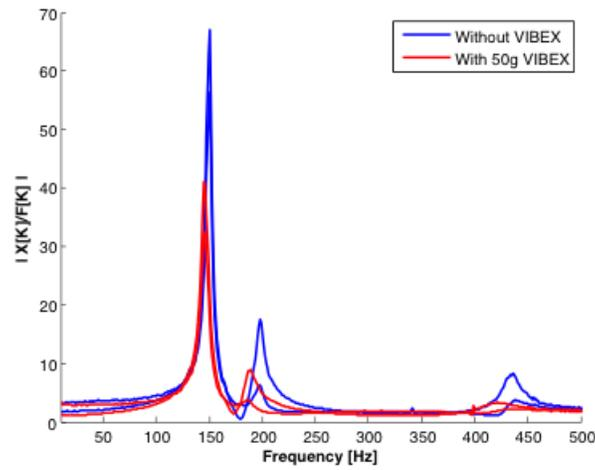
Figure 9: FFT of all Sensors (Impact location – 2, at the front end of the holder)
