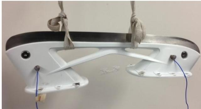
Figure 3: Easton Mako CXN blade holder suspended with accelerometers
