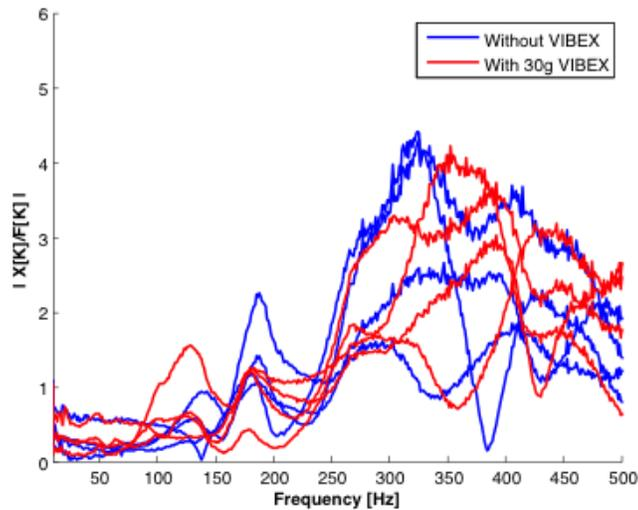
Figure 7: FFT of all Sensors from the entire skate (Impact at boot toe box)
