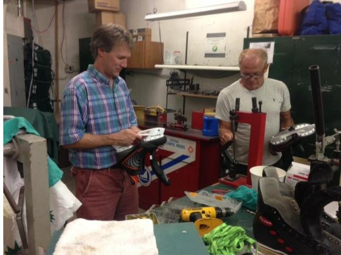
Figure 5: Brian and Tom in the workshop with Easton Mako CXN skates (riveting the holder and grinding the blade profile)
