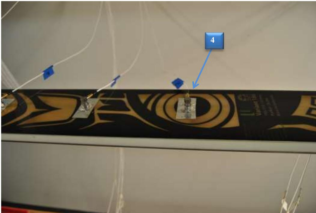
Picture 4: A cavity filled with VIBEX HP (Location #1 at 285mm)
