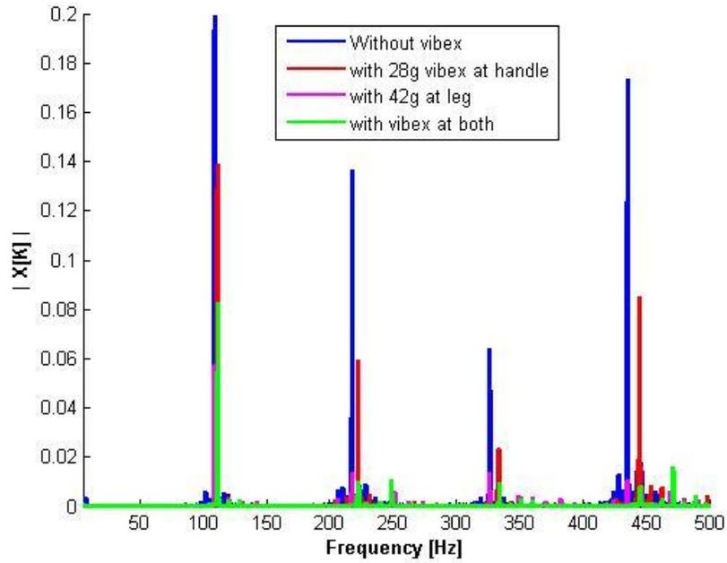
Figure 4. FFT of all sensors during operation of the line trimmer
