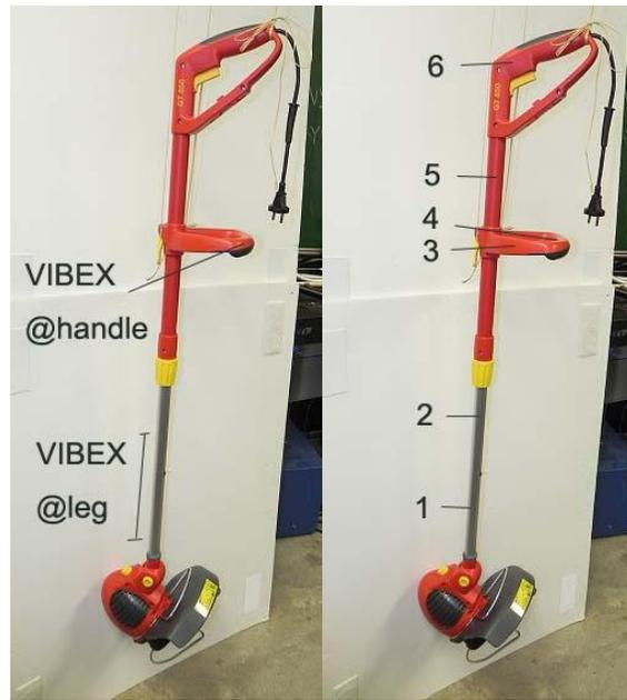
Figure 1: (left) VIBEX locations and (right) sensor locations for the line trimmer
