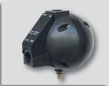
The external automatic drain valve is used larger amounts of condensate (up to 300l/h) must be automatically discharged from filters, pressure vessels and cyclone separators. It ensures reliable operating up to 20 bar. When the condensate exceeds the discharge level, the float rises, opens the discharge aperture and discharges condensate from the system. No power supply required.
